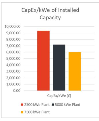
The graph above illustrates the entity of the decrease. The price/kWe installed of large digestion sites improves as the size of the installation increases. In order to reap the benefit of economies of scale, adequate amounts of feedstock need to be available on a daily basis. As explained in the previous section, the availability of large quantities of feedstock can be enhanced by transporting the feedstock from nearby locations.
